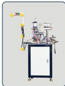
2 SYM-104NA-U 尼龙全自动超声波U型上止机 Nylon fully automatic ultrasonic U type top stop machine
