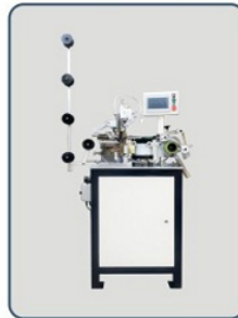
3 SYM-104MA-U 金属全自动U型颗粒上止机 Metal fully automatic U particles top stop machine
