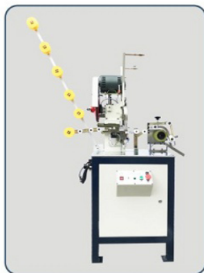
6A SYM-104NA 尼龙全自动上止机 Nylon fully automatic top stop machine
