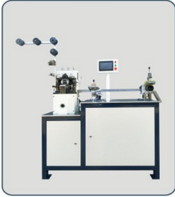
SYM-100IA 隐形全自动免修齿定寸机 Plastic teeth fully automatic CNC gapping machine
