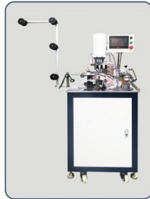
SYM-104IA-U 隐形全自动超声波U型上止机 Stealth fully automatic ultrasonic U type top stop machine
