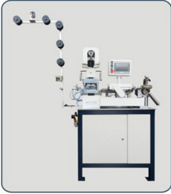
SYM-100DA 胶牙全自动数控定寸机 Plastic teeth fully automatic CNC gapping machine
