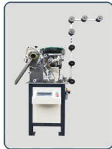
2 SYM-2A 全自动穿头机 Fully automatic wear head machine
